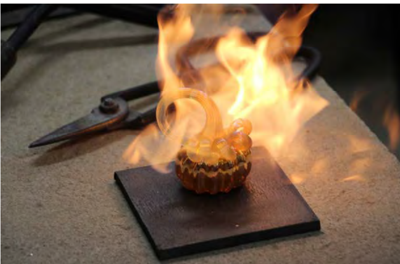
A torch is used to keep the piece hot while working on the stem.
