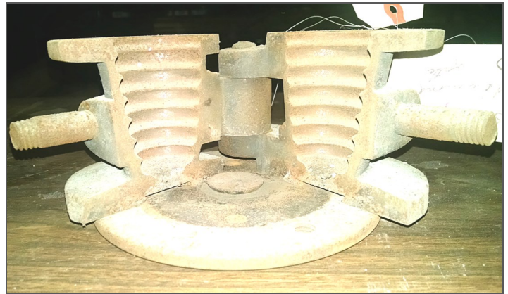
Fig. 4. Blown Saturn Optic mould, opened
