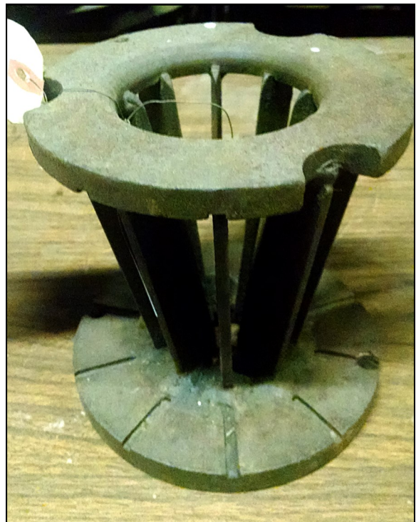
Fig. 7. Wide Optic mould with ten divisions
