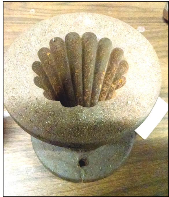
Fig. 6. Medium Optic mould; 14 flutes become 14 panels in the finished product
