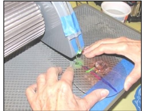
sawing the glass
