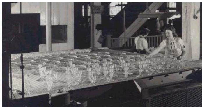
Women at the Heisey factory remove glass from the endless belt as the pieces exit the Lehr.
