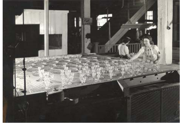
Inspecting glass off the lehr
