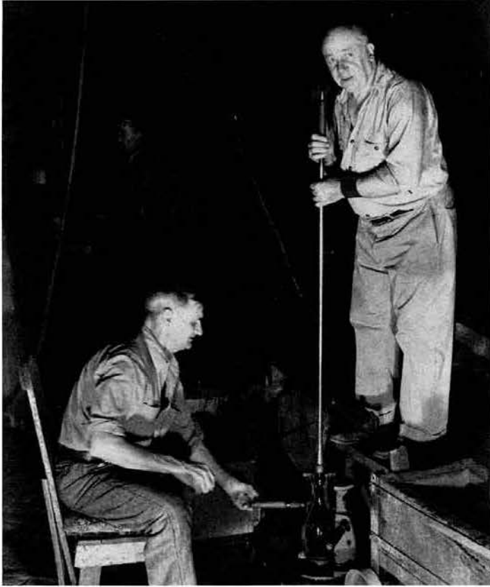
This photo depicts a blower just as he has finished blowing his piece in the mold. His assistant is opening the mold, so that the piece may be removed and taken to another worker for the next step.
