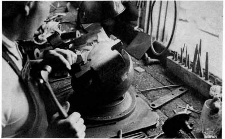
Moldmaker chiseling out a candlestick mold.
