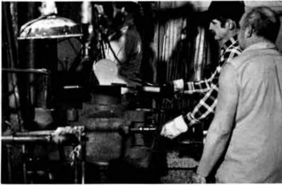
Workers pouring molten glass into the mold.
