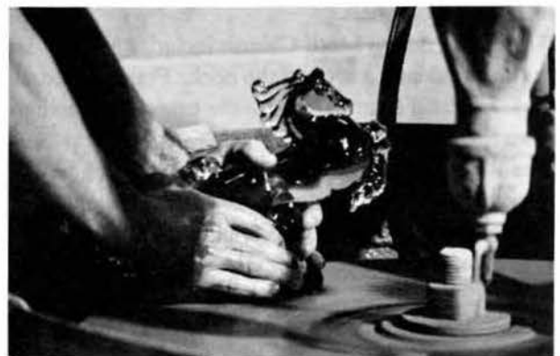
Grinding base of Flying Mare on sandstone grinder.
