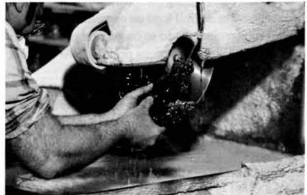
Removing bust-off with saw.
