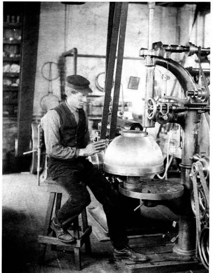
Mr. Ingler making a mould for a 2001 Hemisphere shade. This is in the Heisey factory.
