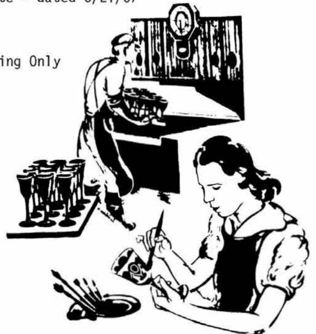
PAINING WAX ON A GOBLET TO BE ETCHED
