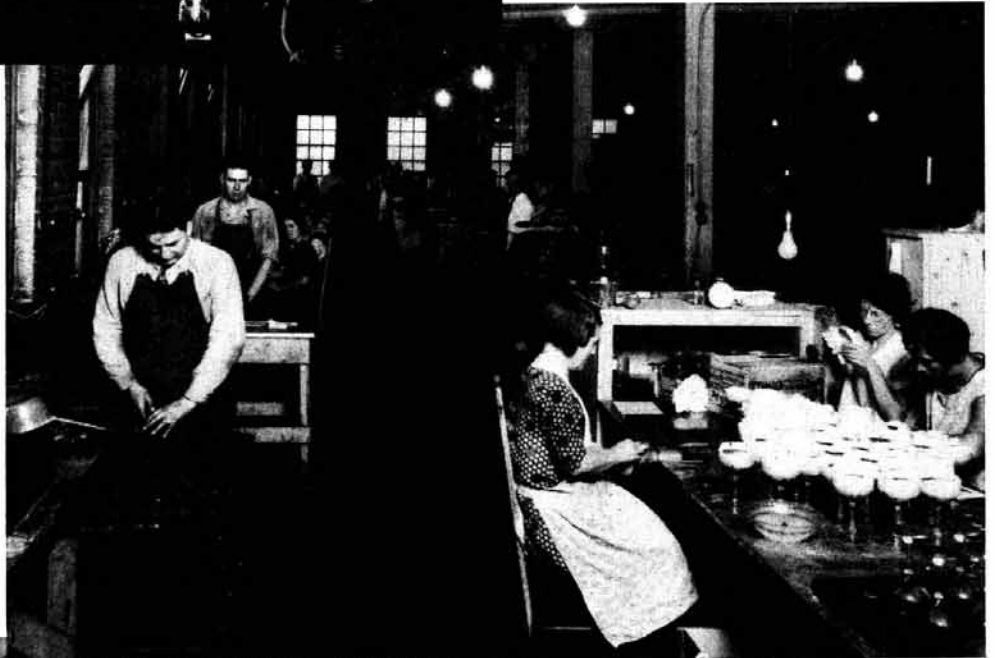
SECTION OF ETCHING ROOM. SHOWS BLACK WAX BEING APPLIED TO DESIGN PLATE - ALSO BEING APPLIED TO GOBLET.
