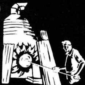
Re-heating and Fire Polishing in "The Glory Hole"
