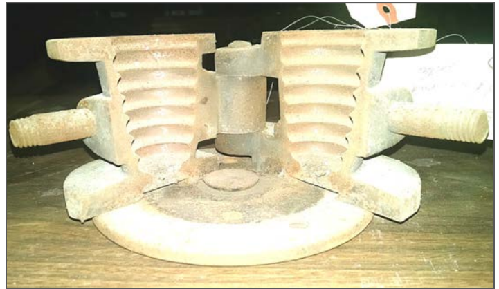
Fig. 4. Blown Saturn Optic mould, opened
