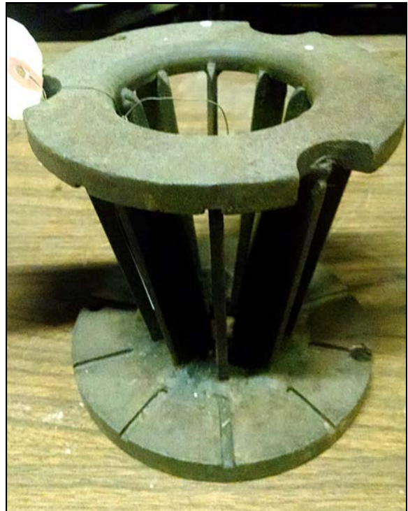
Fig. 7. Wide Optic mould with ten divisions
